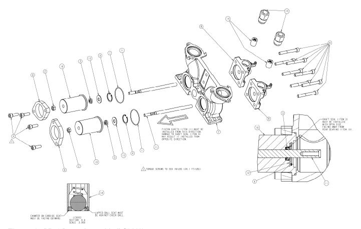
Figure 46: PR70 Pump Assembly (LC0112)
